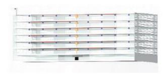
Axell Wireless' D-MBR repeater is powerful enough to drive a passive Distributed Antenna system (DAS) for coverage areas over 10,000m2 in buildings, parking lots, malls, warehouses and offices.
